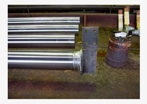
Therefore it is more usual to plate tubes for the full length. But if un-plated areas are required this can be produced.
