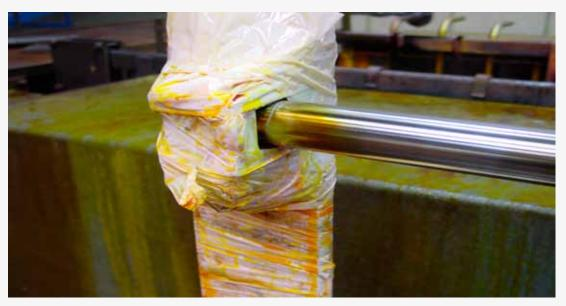
This illustration is a piece of 45mm Chrome Bar and would have un-plated ends no greater than 50mm in length.
